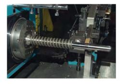
Using the latest in CNC coiling technology, springs are produced with much better predictability and consistency in performance, rates and lengths.
