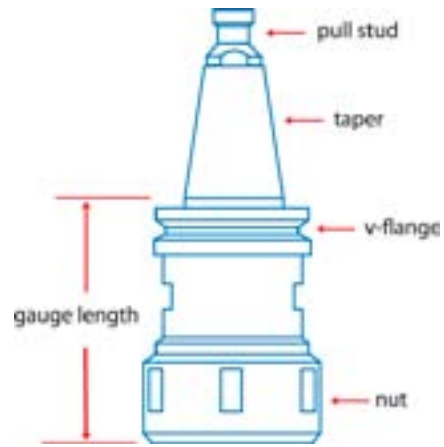
Parts of a collet and nut style toolholder
