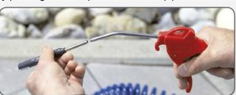
**Step 3:** Blow air through the lead pipe from both sides, if available use compressed air.
