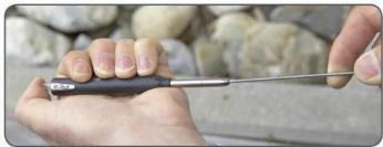
**Step 1:** Press out the stuck lead with a long pin from the front end. At the same time open the mechanism by pushing the transparent lead feed pipe.
