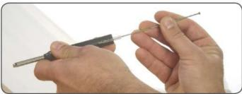
**Step 2:** If step 1 did not work, try to press out the stuck lead with a long pin from the back end which may take quite high force.
