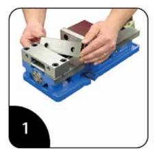
**Step 1** Remove stationary jaw plate.
