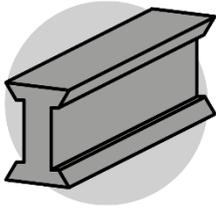
Hard materials, including hardened steel, alloy steel or cast iron, are tougher to drill than soft materials. A tool with correct power, torque and speed is imperative for drilling hard materials. Lower speed and lubrication are success factors here!
