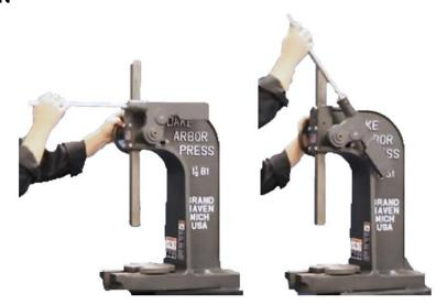
CAUTION: NEVER PULL THE PRESS HANDLE PAST THE HORIZONTAL POSITION! To avoid personal injury and damaging the press only pull until the handle is horizontal, then return the handle back up as far as it allows before bringing the handle back down. This ensures that the pawl fully engages with the gear teeth to prevent tooth damage and gear slippage that can cause harm to the machine and worker. Examples above show the proper minimum and maximum handle positions.
