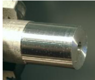
Workpiece after turning with power feed
