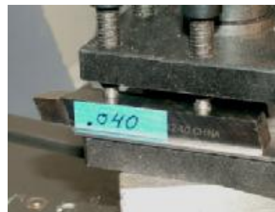
Tool bit height adjusted by shims
