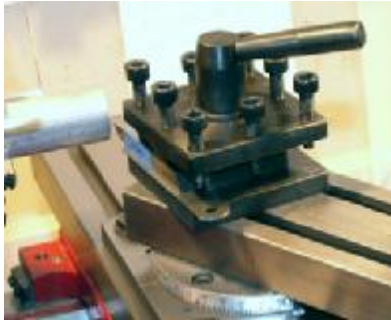
Tool positioned for a facing cut
