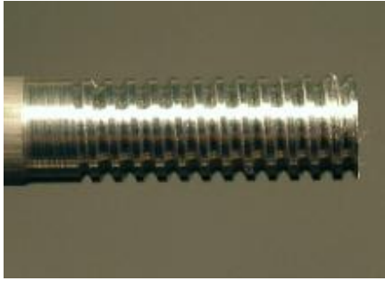
Thread gets deeper on each pass
