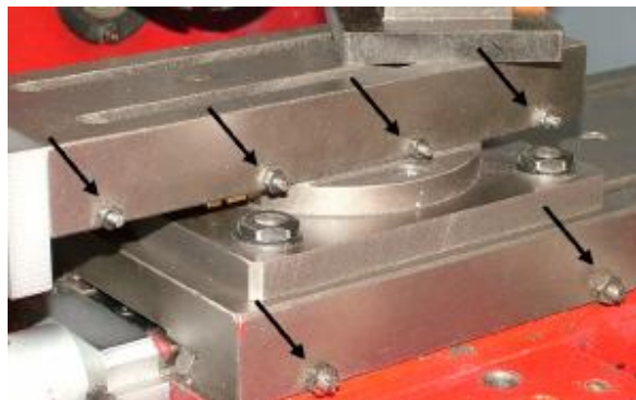
gib adjustment screws
