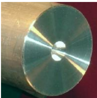
Completed center-drilled hole
