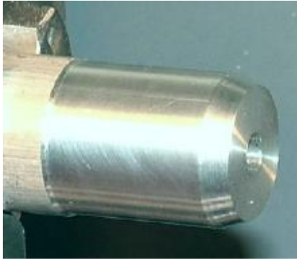
Completed bevel cut
