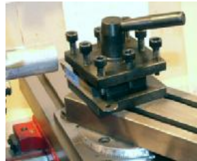
Tool positioned for a facing cut
