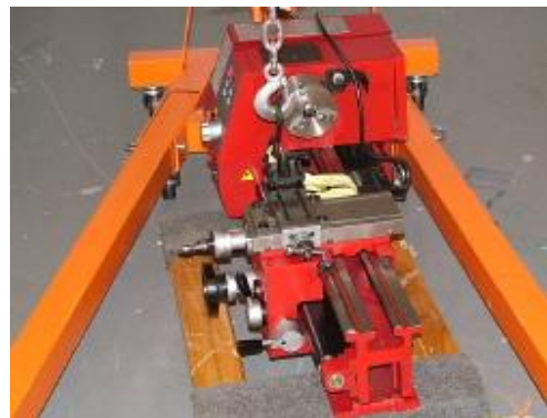
Using a shop crane to lift the lathe
