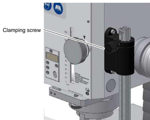
Fig. 1-5: Separating protective equipment
