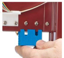
The second clip is holding the Z-axis arm down. Gently lift the X-axis arm a few inches. Do not lift the arm by the platform as this may affect the levelling of the platform!
