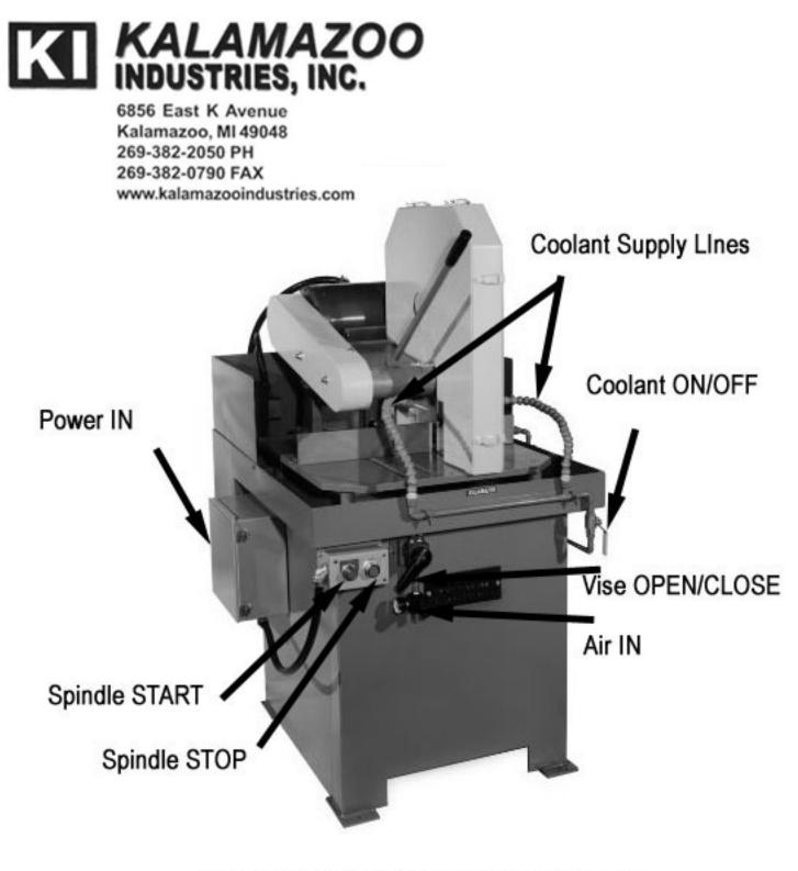
Model: K20SW 20" dia. wet abrasive saw Table Dims: 27"w x 30"deep
