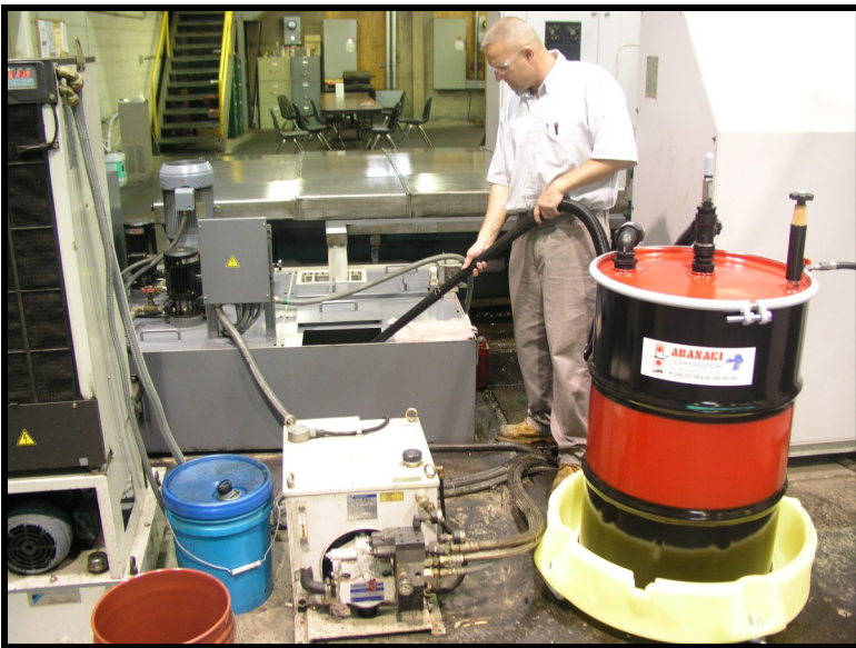
Gary Ott at Hahn Manufacturing uses the Chiperator to clean out a sump.
